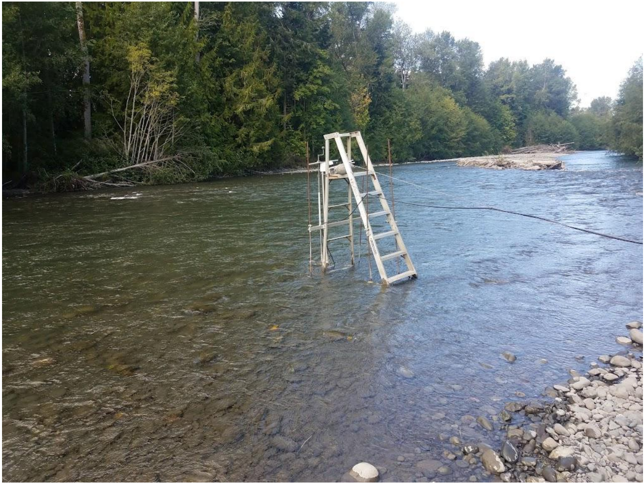
Figure 3. "Old OM SONAR site". The SONAR was operational in this location from July 9 through September 23, 2025. The SONAR is attached to the pole mount which is in turn attached to the ladder. The river is moving from left to right.
